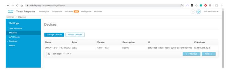
You can associate this device to a module, navigate to **Modules > Add New Module > Web Security Appliance**, as shown in the image.
