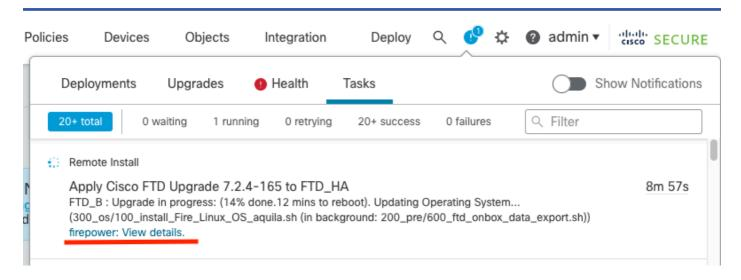
If you click on **firepower: View details**, the progress is shown in a graphical way and the logs of status.log.
