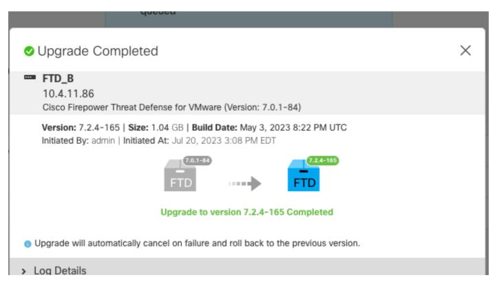
After the upgrade is completed in the Standby device, it starts in the Active device.
