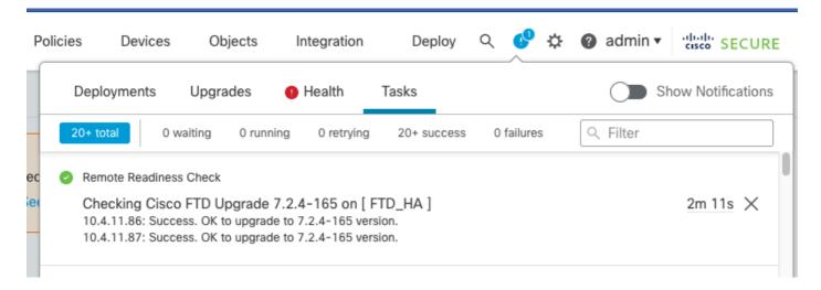
When the readiness check completes in both FTD and result is Success, the upgrade can be done.
