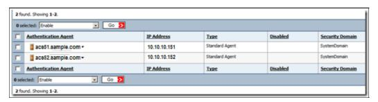
4. In the RSA Security Console, navigate to *Access > Authentication Agents > Generate Configuration File* in order to generate the sdconf.rec configuration file:
