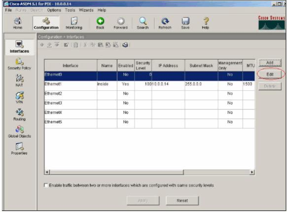
2. Check **Enable Interface** and enter the Interface Name and Security Level for the interface. Choose **Obtain address via DHCP** for the IP address and **Obtain default route using DHCP** for the default gateway and then click **OK** to go to the Main window.
