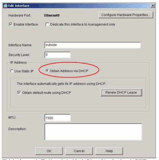
3. Click **Apply** to see the IP address obtained for the Ethernet0 interface from the DHCP server.
