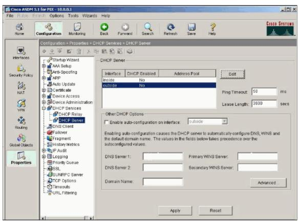
2. Check **Enable DHCP server** on the outside interface to listen for the requests of the DHCP clients. Provide the pool of addresses to be issued to the DHCP client and click **OK** to return to the Main window.
