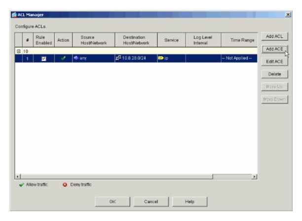
In this example, a second ACE is added to ACL 10 in order to permit access to the Intranet subnet.
