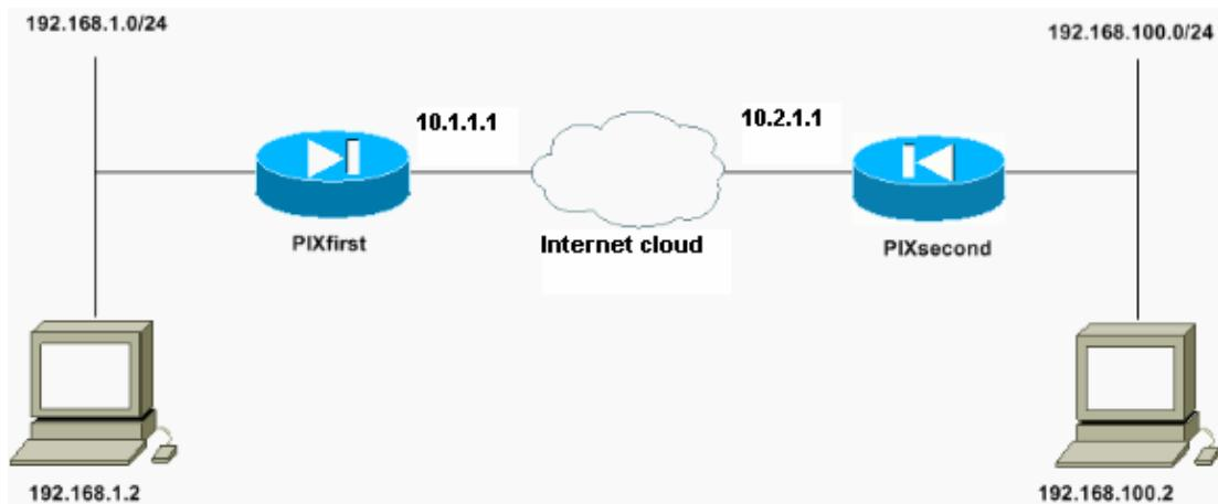
The host with the IP address of 192.168.100.2 is translated to 192.168.50.2 on the PIX Firewall with the host name of PIXfirst. This translation is transparent to the host and its destination.
