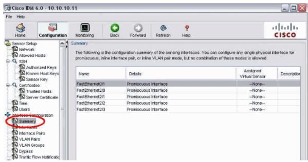
6. Go to Configuration > Interface Configuration > Interfaces and select the interface name. Then, click Enable in order to enable the sensing interface. Also, configure the Duplex, Speed and VLAN information.
