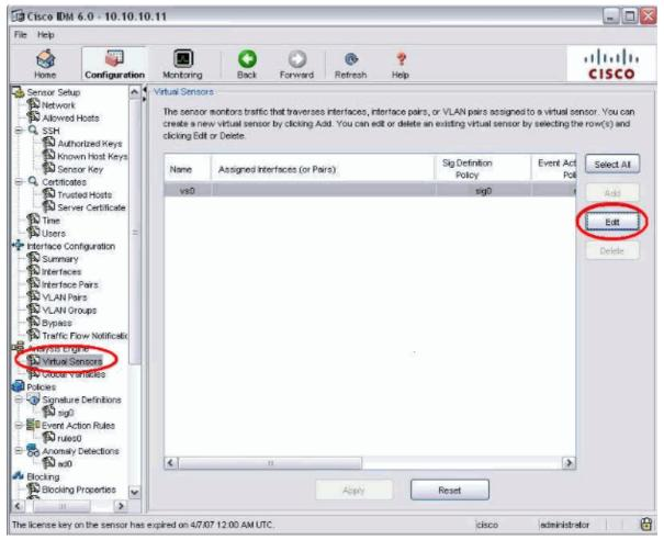
10. Assign the Inline pair **INLINE** to the Virtual Sensor vs0.
