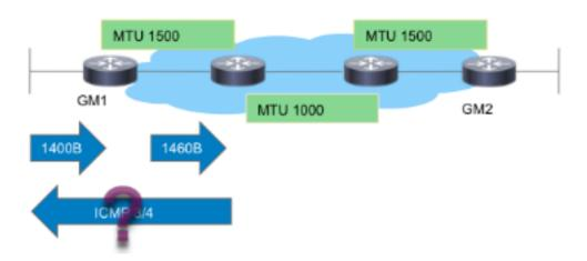
As the image shows, PMTUD breaks down with GETVPN with this flow:
