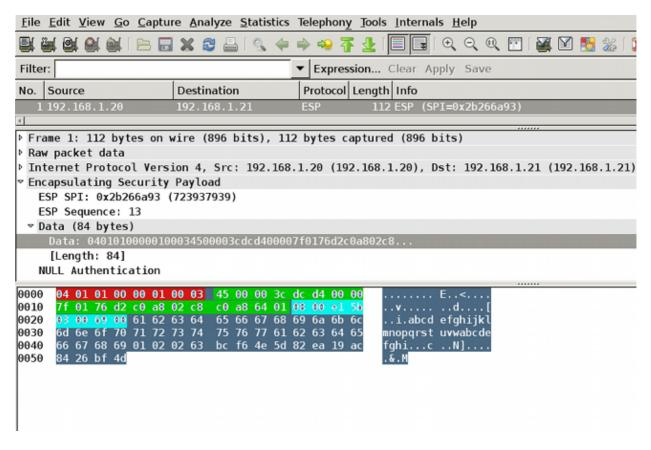
Wireshark has been used to decode null encryption for the security parameter index (SPI). In the IPv4 header, the source and destination IP are the Internet IP addresses of the routers (used as tunnel source and destination).
