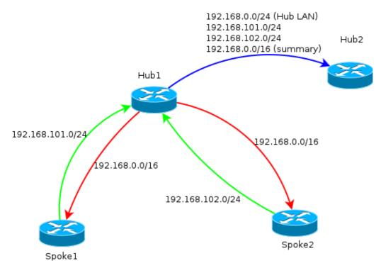
*Note*: In the diagram, the green line represents information provided by spokes to the hub, the red line represents information provided by each hub to the spokes (a summary only), and the blue line represents prefixes exchanged between hubs.
