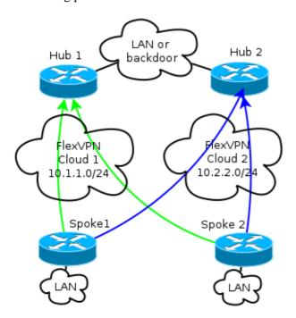
*Note*: In the diagram, the green lines show the connection and direction of Internet Key Exchange Version 2 (IKEv2)/Flex sessions to Hub 1, and the blue lines indicate the connection to Hub 2.
