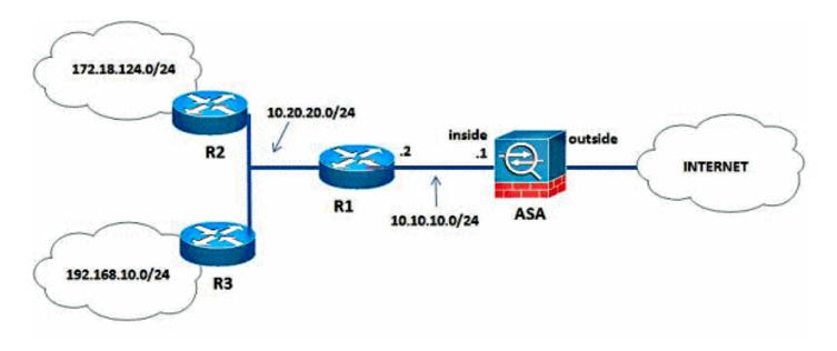
In the network topology that is illustrated, the Cisco ASA inside interface IP address is 10.10.10.1/24. The goal is to configure EIGRP on the Cisco ASA in order to learn routes to the internal networks (10.20.20.0/24, 172.18.124.0/24, and 192.168.10.0/24) dynamically through the adjacent router (R1). R1 learns the routes to remote internal networks through the other two routers (R2 and R3).
