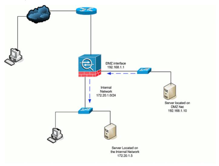
1. Create a static NAT entry for the AD/DNS server on the DMZ. Static NAT creates a fixed
