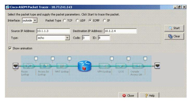
The packet-tracer output with the **same-security-traffic permit intra-interface** command enabled and the **access-list outside\_acl extended deny ip any any** command configured to deny packets.
