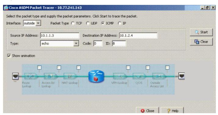
The packet-tracer output with the **same-security-traffic permit intra-interface** command disabled.
