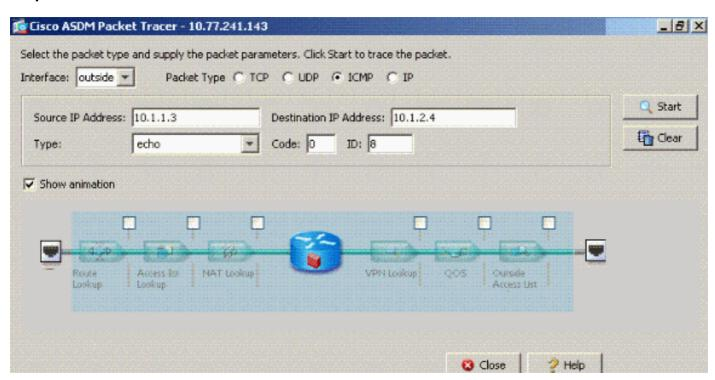
The packet-tracer output with the **same-security-traffic permit intra-interface** command enabled and the **access-list outside\_acl extended deny ip any any** command configured on the same interface where intra-interface traffic is desired.
