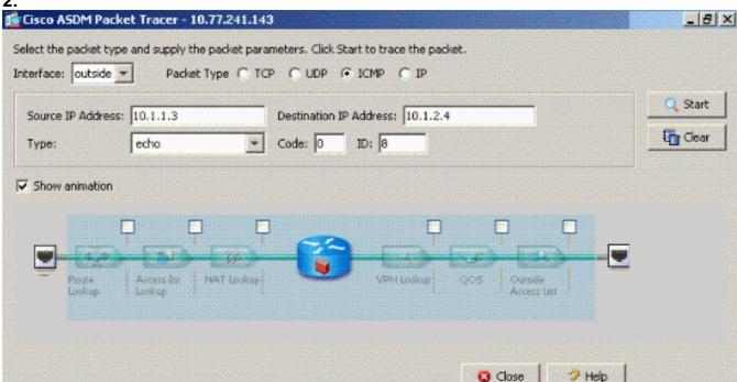
The <u>packet-tracer</u> output with the **same-security-traffic permit intra-interface** command enabled.
