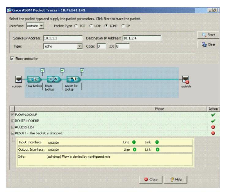
The packet-tracer output <code>drop...implicit rule</code> suggests that a default configuration setting is blocking the traffic. The administrator needs to check the running configuration in order to ensure intra-interface communications are enabled. In this case, the ASA configuration needs intra-interface communications to be enabled (<code>same-security-traffic permit intra-interface</code>).
