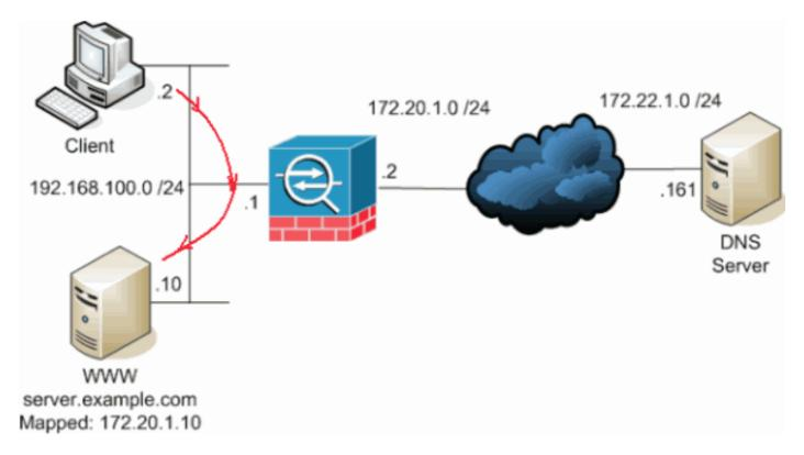
In this case, the client at 192.168.100.2 wants to use the public address of the WWW server (for example, 172.20.1.10). The DNS services for the client are provided by the external DNS server at 172.22.1.161. Because the DNS server is located on another public network, it does not know the private IP address of the WWW server. Instead, the DNS server knows the WWW server mapped address of 172.20.1.10.
