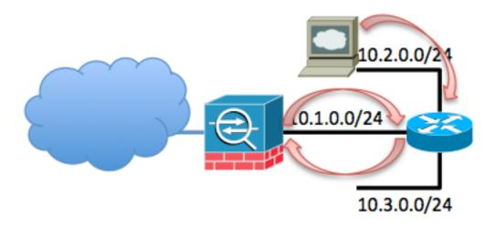
This loop occurs until the TTL of this packet decrements to 0. Note that the ASA Firewall **does not** decrement the TTL value by default when it processes a packet. The router decrements the TTL as it routes the packet. This prevents the occurrence of this loop indefinitely, but this loop does increase the traffic load on the ASA and causes the CPU usage to spike.
