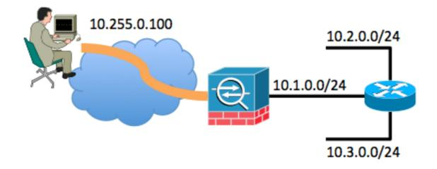
In this example, the remote access client has been assigned the IP address of 10.255.0.100. The ASA in this example is connected to the same inside network segment along with a router. The router has two additional Layer 3 network segments connected to it. The relevant interface
