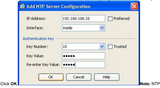
Server details should be specified within the context System. However, since the System Execution Space does not include any interfaces in multiple context mode, you need to specify an interface name (that is, defined within the Admin context).
