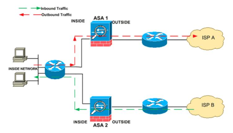
**Note:** TCP state bypass feature is disabled by default on the Cisco ASA 5500 Series Adaptive Security Appliances.
