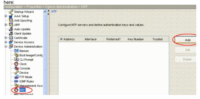
3. Click the ADD button in order to add a NTP server and provide the required attributes such as IP address, Interface name (Inside or Outside), key number and key value for Authetication in the new window that comes up after you have clicked on the ADD button as shown in the screen shot. Then click on
