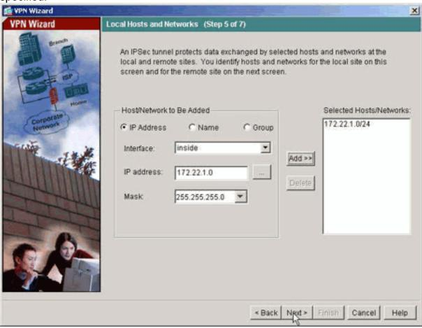
11. The hosts and networks on the remote side of the tunnel are specified.
