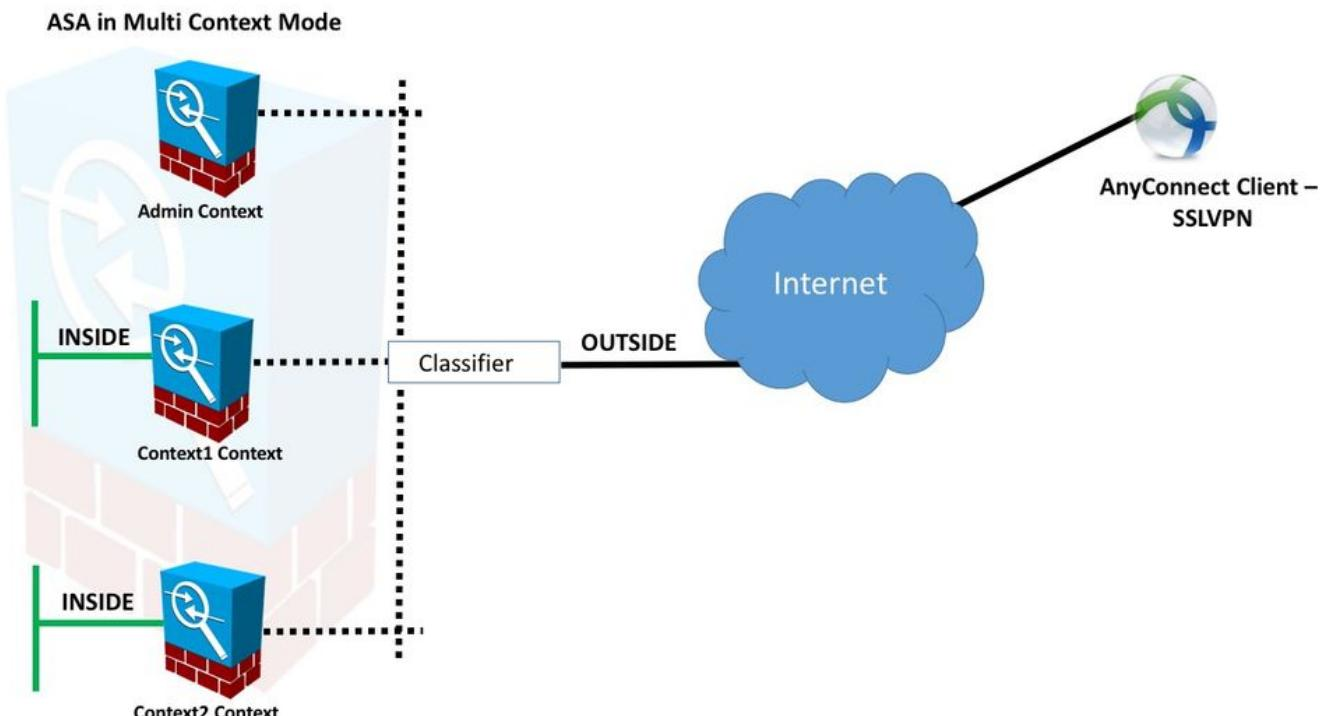
**Note:** Multiple contexts in this example share an interface (OUTSIDE), then the classifier uses the interface unique (auto or manual) MAC addresses to forward packets. For more details on how security appliance classifies packets in multiple context refer [How the ASA Classifies Packets](#)
