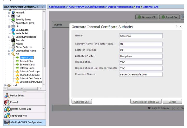
Click on **Generate self-signed CA** to generate the internal CA certificate. Then click on **Generate CSR** to generate the certificate-signing-request which is consequently shared with the CA server to sign.
