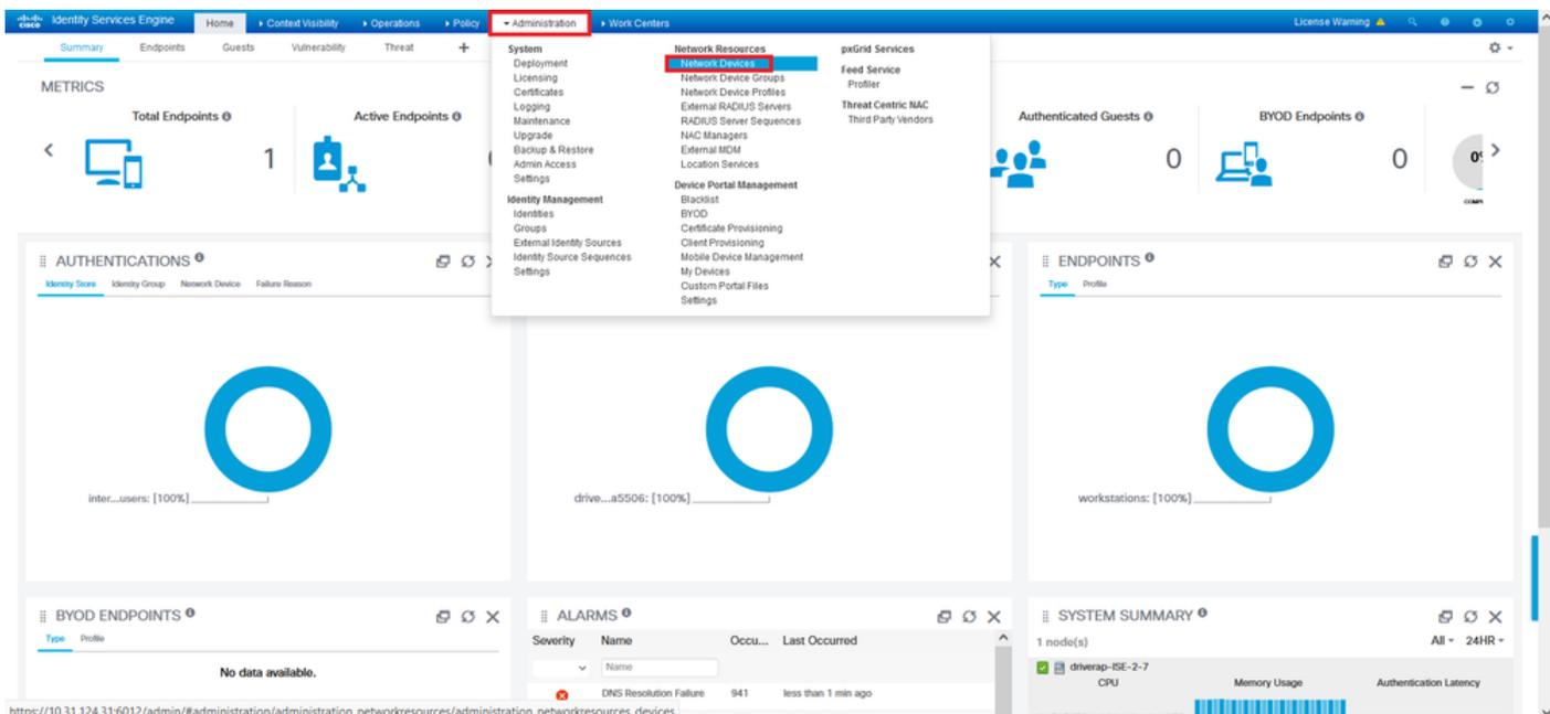
Step 2. In the Network Devices section, click **Add** so ISE can process RADIUS Access Requests from the FTD.
