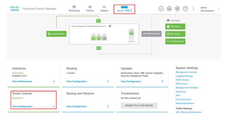
2. Verify that the FTD is registered to the smart licensing server and that the AnyConnect Plux, Apex, or VPN Only license is enabled.
