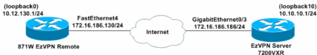
**Note:** Loopback interfaces are simulating the inside PCs.
