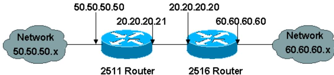
Here are configurations for two routers (a Cisco 2511 and a Cisco 2516) back-to-back doing IPSec and ISAKMP authentication based on a preshared key. Comment lines are indicated by an exclamation point as the first character and are ignored if entered into the router. In the configuration below, comments precede certain configuration lines in order to describe them.
