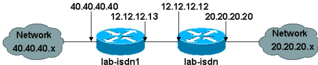
The sample configuration below is taken from two Cisco 1600 routers that have previously obtained CA certificates (as shown above) and intend to do ISAKMP with "rsa-sig" as the authentication policy. Only traffic between the two remote Ethernet LANs is encrypted.
