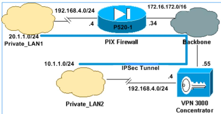
Both Private\_LAN1 and Private\_LAN2 have an IP subnet of 192.168.4.0/24. This simulates the overlapping address space behind each side of the IPSec tunnel. The VPN 3000 Concentrator is used here as one example of a concentrator which does not have the functionality of NAT over VPN traffic.
