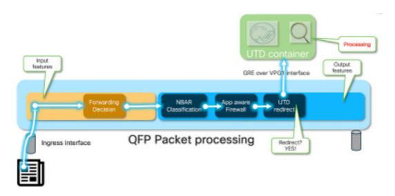
Traffic comes from the LAN side. Since IOS® XE knows the container is in a healthy state, it diverts the traffic to the UTD container. The diversion uses the VirtualPortGroup1 interface as the egress interface, which encapsulates the packet inside of a Generic Routing Encapsulation (GRE) tunnel.
