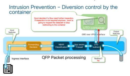
For instance, with HTTPS flow, the preprocessors are interested to see the server Hello / Client Hello packets with TLS negotiation. Afterwards the flow is not redirected since there is little value in inspecting TLS encrypted traffic.
