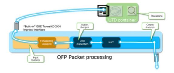
Container controls the diversion result in the UTD inspection in the IOS® XE datapath.
