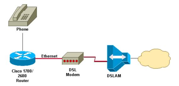
You can apply a hierarchical policymap (see the PPPoE configuration) to the Ethernet interface where PPPoE is enabled. Ensure you configure the correct speed for the shaping. For example, in the DSL environment, if your upstream limit is 128 kbps, you should shape to 128 kbps.
