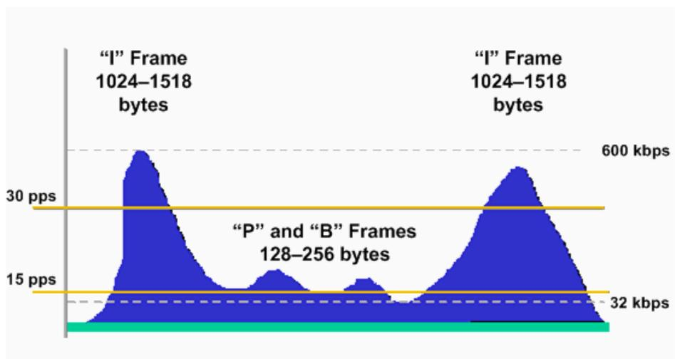
The "I" frame is a full sample of the video. The "P" and "B" frames use quantization via motion vectors and prediction algorithms.
