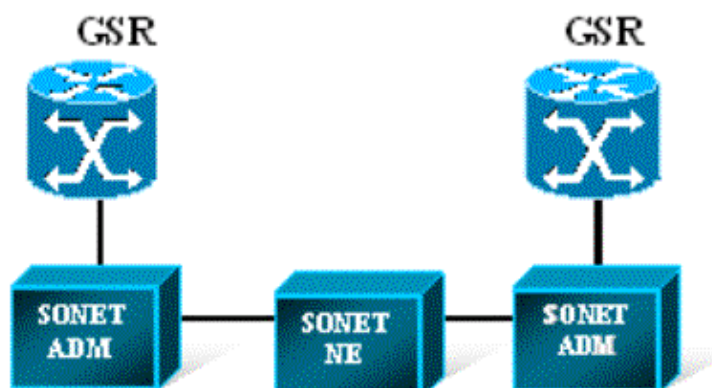
Figure 4 POS Connection Over a SONET Network
