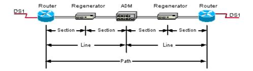
When you connect two router POS interfaces point to point, over a dense wavelength division multiplexing (DWDM) link without intermediate SONET or Synchronous Digital Hierarchy (SDH) equipment, all three BIP mechanisms monitor the same segment, and typically detect the same errors. However, in this configuration, B2 must provide the most accurate bit error count.
