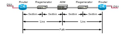
At the source node, the path layer (PTE) maps 28 DS1 signals and path overhead to form an STS-1 Synchronous Payload Envelope (SPE) and hands this to the line layer.
