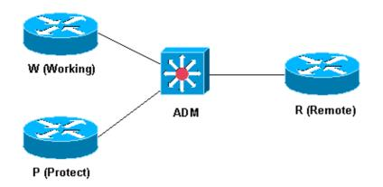
W and P each transmit a distinctive identifying signature in the path overhead of the standard SONET or Synchronous Digital Hierarchy (SDH) frame. R reflects it back in a different part of the path overhead.
