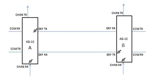
From the diagram, you can understand that you have VOAs on EXP-TX and CHAN-RX ports, and the same applies to all other types of cards. In the ANS parameter, you have a set point of COM-RX and COM-TX.
