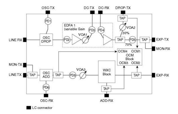
As shown in this diagram, there is no amplifier unit between the EXP-RX and the LINE-TX port. The Line-TX port transmits the optical power received on the EXP-RX port.
