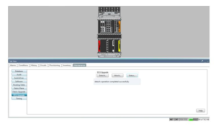
Once the alarm is cleared, the ECU Module can be physically removed.
