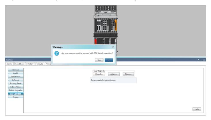
Step 1.6.c. In alarms, 'The detach provision for disk started' and 'disk provision in progress' minor alarm will appear.
