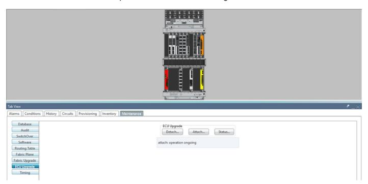
Alarm 'The attach provision for disk started' will be raised once the attach procedure is triggered.
