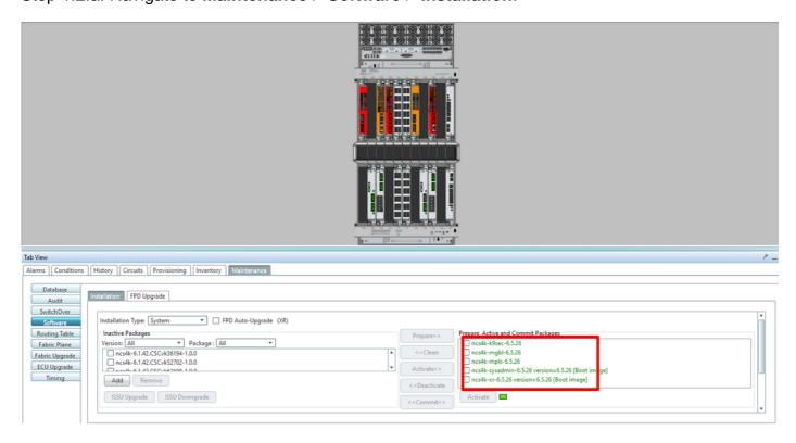
Step 1.2.b. The software must be minimum of 6.5.26 software in order to complete this procedure.
