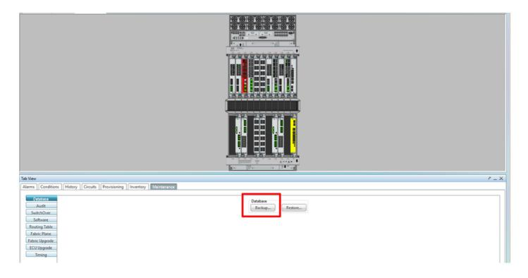
Step 1.4.c. Select/Enter the full path with the file name in order to save the backup on the node.
