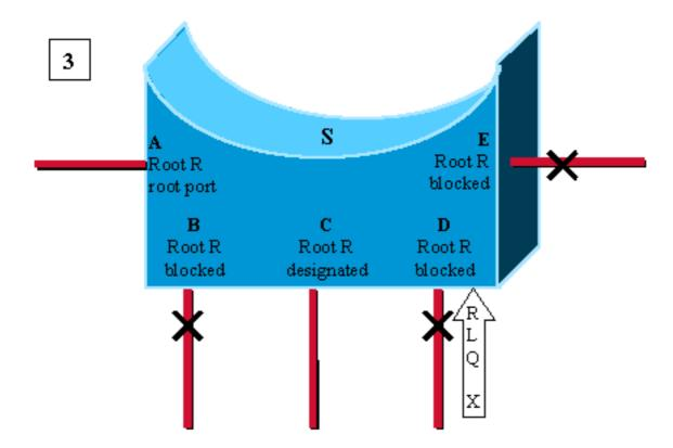
Port D is the first to receive and RLQ response from bridge X claiming to be the root. It is a negative response: D has lost connectivity to the root R. We age out immediately the BPDU on port D and go to listening. As we don't know if we still have connectivity to the root R, we don't age out port E yet.
