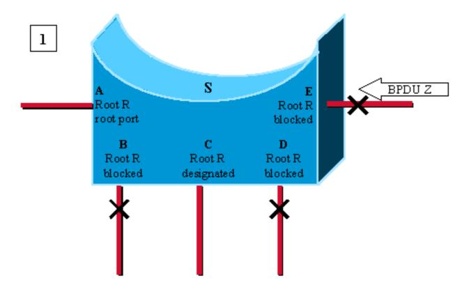
Port E receives an inferior BPDU, advertising root Z instead of root R stored on the different ports.
