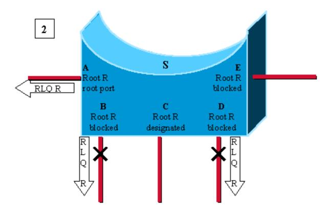
Switch S needs to recheck all its other non-designated ports. It sends out a RLQ request for root R on ports A,B and D.
