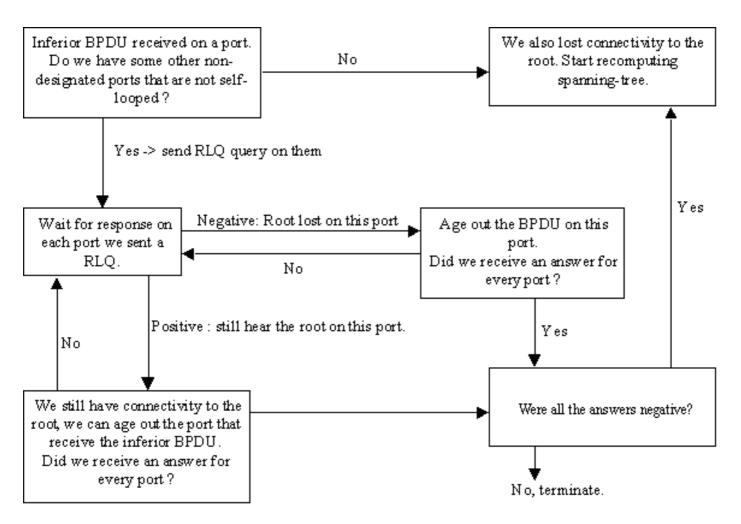
On receipt of an inferior BPDU from a designated bridge, send a RLQ PDU on all non-designated ports except the port where you received the inferior BPDU and self-looped ports. This is in order to check that you still hear from the root on ports where you are used to receiving BPDUs. The port where you received the inferior BPDU is excluded because you are already aware that it suffered from a failure, self-looped and designated ports are not useful, as they do not lead to the root.
