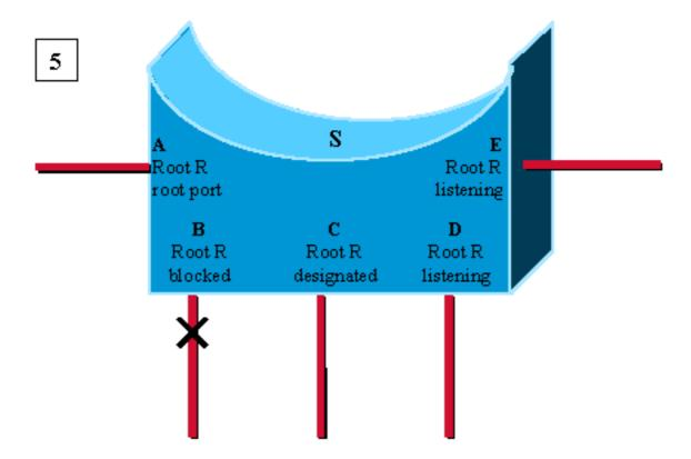
Port E transitions to listering, without waiting for max\_age. Usual spanning-tree rules then apply to determine whether E and D will eventually go to blocking or forwarding.
