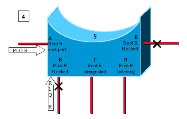
Here, A and B receive a RLQ response confirming R as being the root. As switch S still has connectivity to the root, we can age out immediately the BPDU stored on port E.
