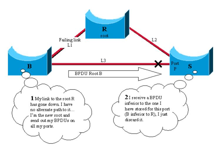
Consider this diagram, which involves three switches R, B, and S in a fully meshed topology. Assume that R is the root bridge and B is the backup root bridge. S blocks its port P and B is the designated bridge for link L3.
