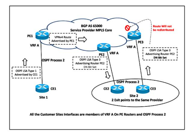
Based on the network topology, PE2 sets the DN Bit for the redistributed LSA and this LSA is never considered for route calculation in OSPF Process 2 on PE3. So PE3 never redistributes this route back into MP–BGP.
