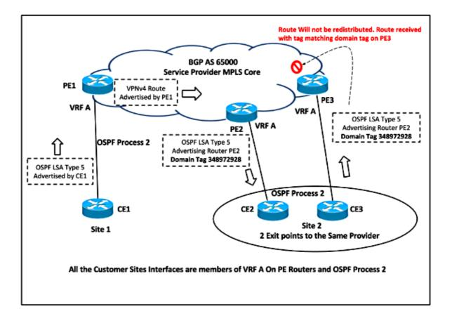
Based on the network topology, PE2 sets the Domain Tag for Type 5 and Type 7 LSA when it redistributes the VPNv4 route into OSPF. This LSA is never considered for route calculation because the DN Bit is already set, but it also has the Domain Tag set, so the LSA is ignored because the Domain Tag matches the VPN / VRF Tag. Hence the route is never redistributed into OSPF.
