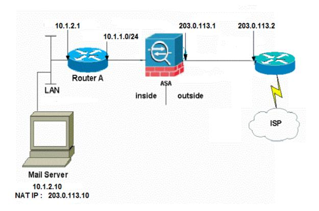
The network setup that is used in this example has the ASA with an inside network at 10.1.1.0/24 and an outside network at 203.0.113.0/24. The mail server with the IP address 10.1.2.10 is located in the inside network.
