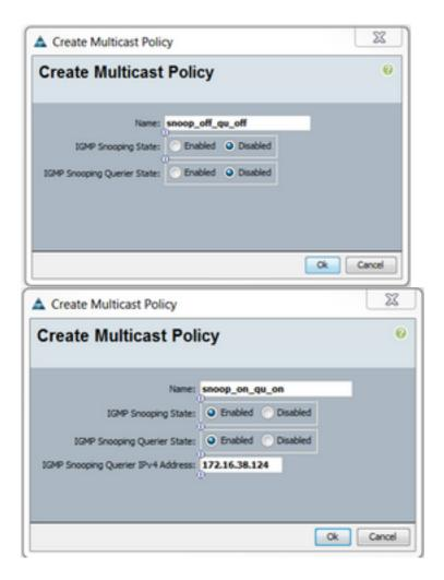
Step 4. If you attempt to disable IGMP Snooping while the IGMP Snooping Querier is enabled, this throws an error, as this isn't a valid configuration.
