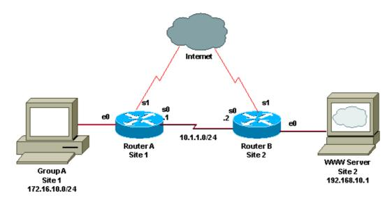
The following is a partial configuration of Router A, showing that a policy route—map called FOO is applied to interface e0, where the traffic from Group A enters the router:
