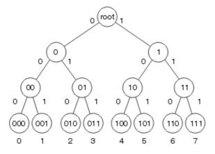
In Fast Switching, the reachability information is indicated by the existence of a node on the binary tree for the destination of the packet. The MAC header and outbound interface for each destination are stored as part of the node's information within the tree. The binary tree can actually have 32 levels (the tree above is extremely abbreviated for the purpose of illustration).
