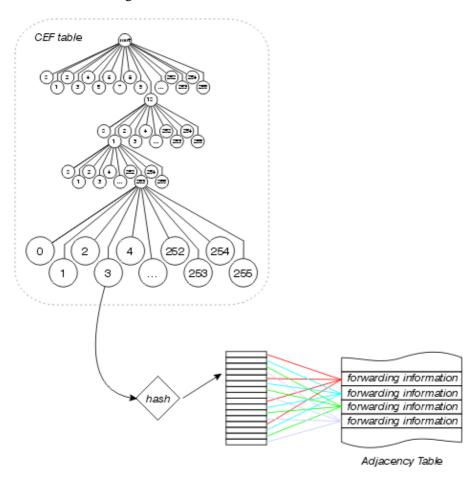
The Cisco Express Forwarding table points to this loadshare table, which contains pointers to the various adjacency table entries for available parallel paths. The source and destination addresses are passed through a hash algorithm to determine which loadshare table entry to use for each packet. Per packet load sharing can be configured, in which case each packet uses a different loadshare table entry.
