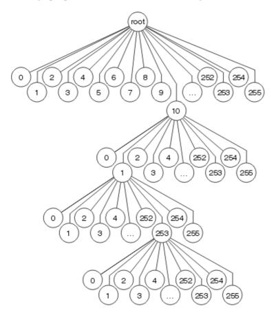
Each octet is used to determine which of the 256 branches to take at each level of the tree, which means there are, at most, 4 lookups involved in finding any destination. For shorter prefix lengths, only one—three lookups may be required. The MAC header rewrite and output interface information are stored as part of the tree node,
