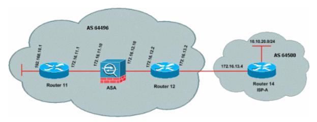
PIX/ASA version 7.x and later introduces an additional challenge when you try to establish a BGP peering session with MD5 authentication. By default, PIX/ASA version 7.x and later rewrites any TCP MD5 option included on a TCP datagram that goes through the device and replaces the option kind, size and value with NOP option bytes. This effectively breaks BGP MD5 authentication, and results in error messages like this on each peering router:
