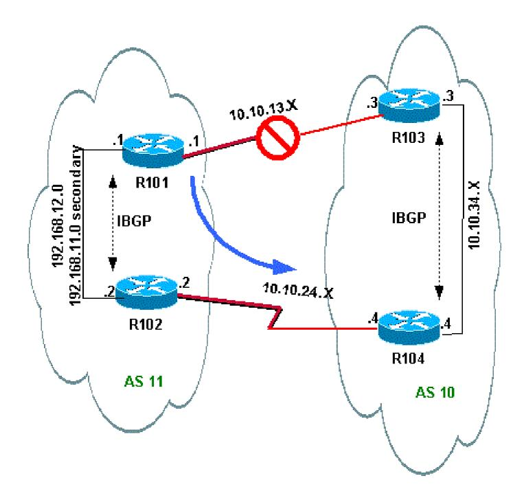
Shut down the R103-R101 link on R103 in order to simulate this situation.
