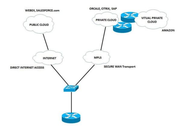
R1 will prefer voice and video traffic to take the best path with a relatively less delay, jitter and/or loss among the two links available to it. Other traffic is load balanced in order to maximize bandwidth.
