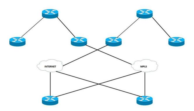
As shown in the diagram, each Branch router is connected to both the providers, one is MPLS which is primary and other is INTERNET which is secondary.
