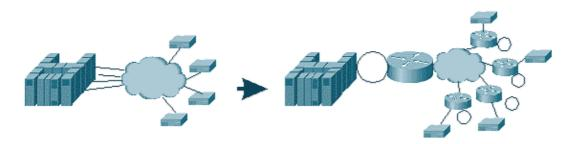
The routers allow the FEP to have only the Token Ring interface. From that point, there are multiple remote locations performing SDLLC to the host, as well as regular source—route bridge (SRB) traffic.
