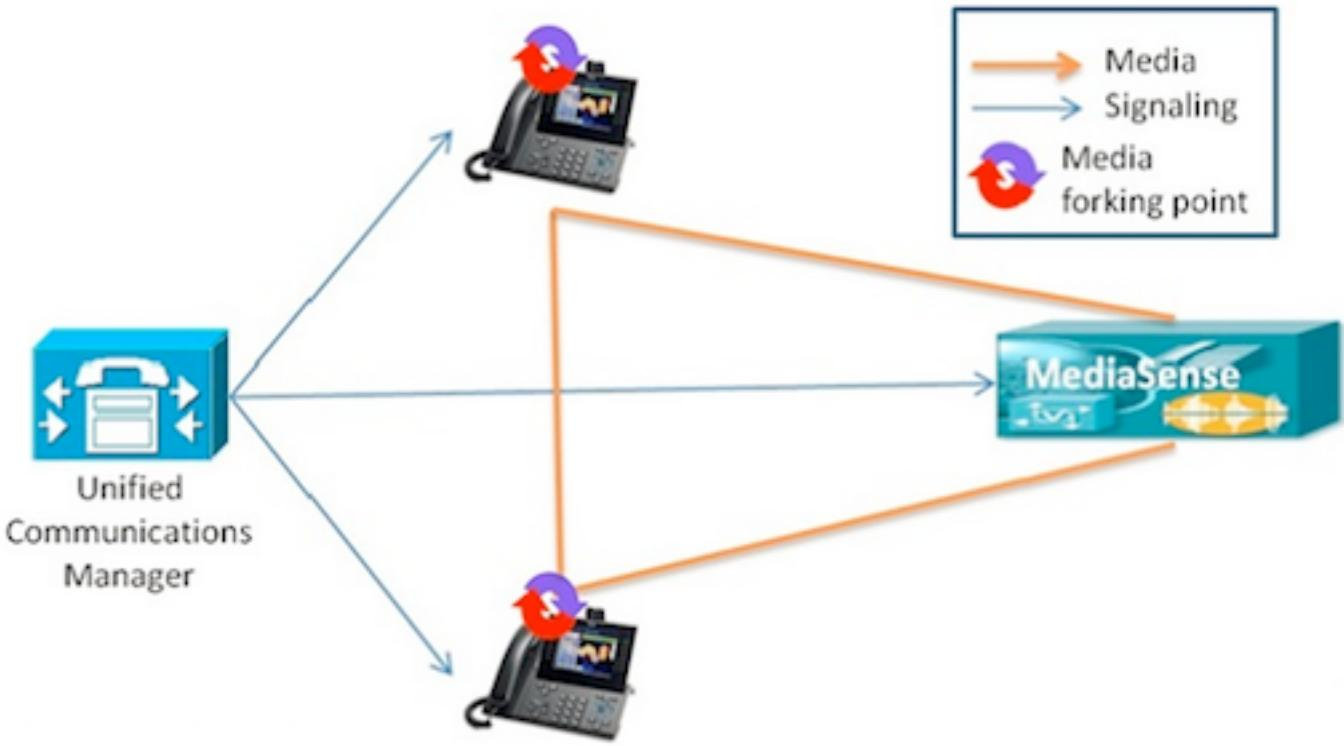
This shows a basic Unified Communications Manager deployment where the call is between internal users who are within the enterprise. It is important that one of the phones be configured for recording. In case both phones are configured for recording, then two separate recording sessions will be captured.
