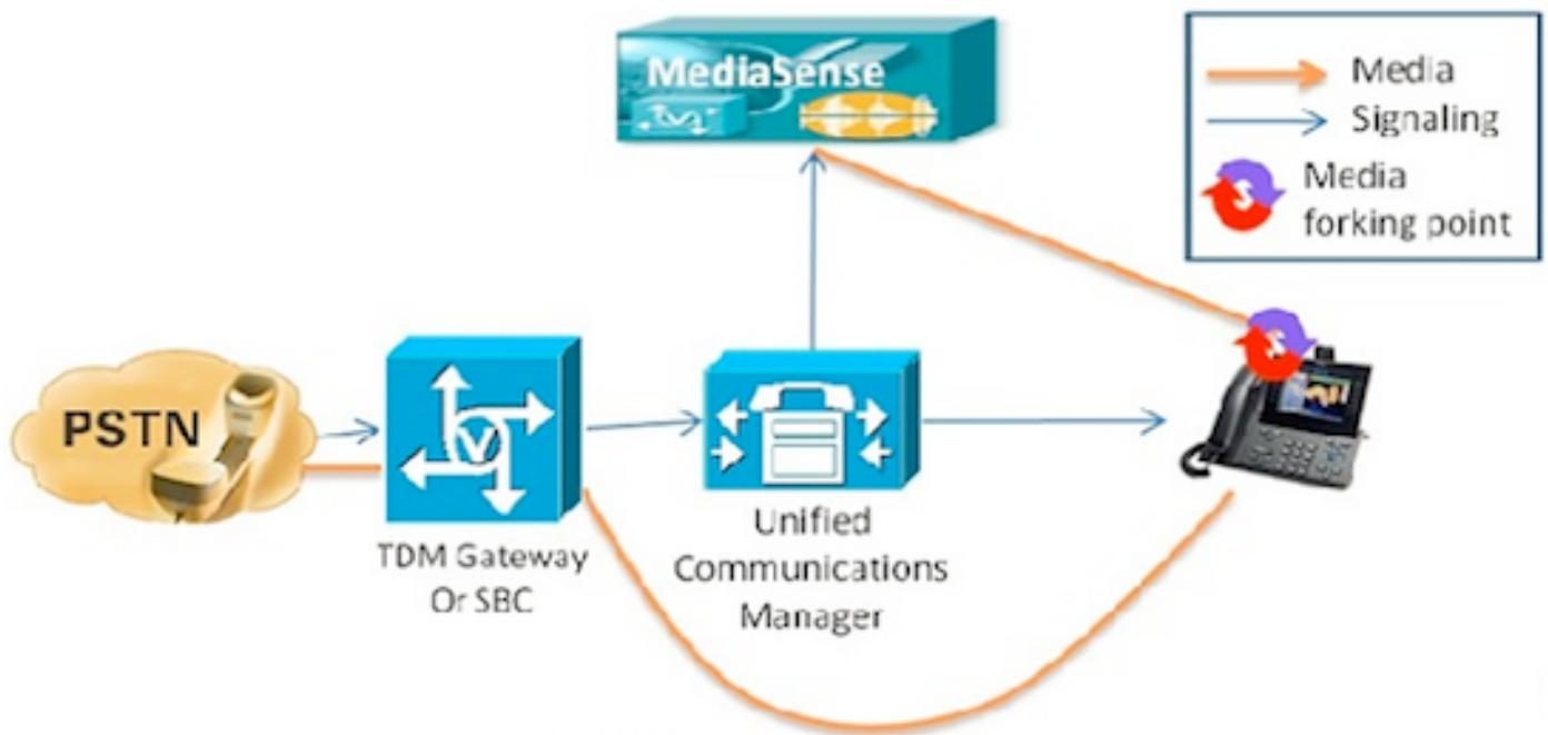
This shows a basic Unified Communications Manager deployment where Cisco IP phone call with an external caller is recorded. This applies to both inbound and outbound calls, as long as the inside phone is configured with an appropriate recording profile.
