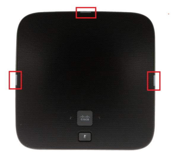
Step 4. Press and hold the MIC button for approximately five seconds, and then release it. The lights should blink red twice.
