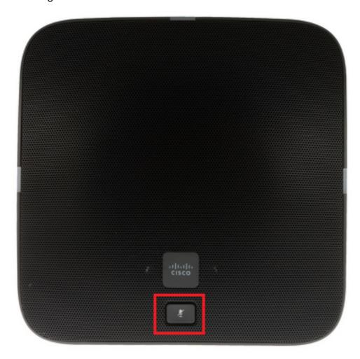
Step 3. Continue to hold the MIC button and power on the phone (plug in the Ethernet cable or the power brick). When the lights that are located on the left, right, and back sides of the phone change from green to red, release the MIC button, as shown in the image.
