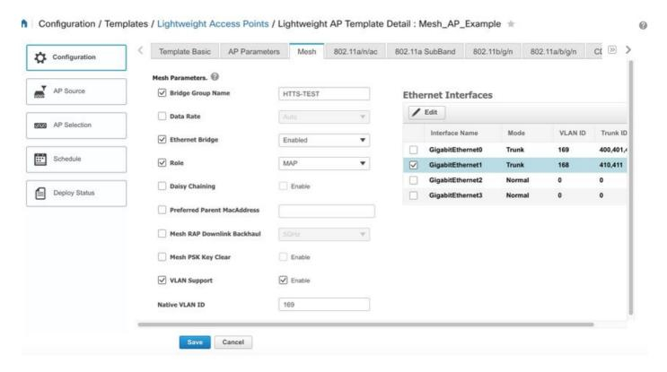
The example shows a RAP with multiple VLAN support and a customised **BGN** named HTTS-TEST.
