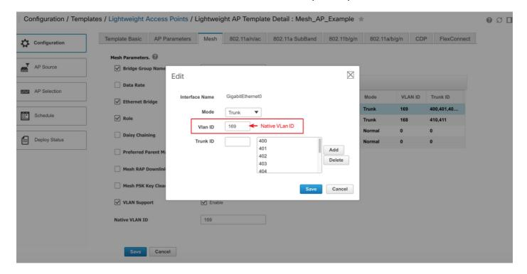
Step 4. Set up CLI Templates for Any Missing Options in Prime Infrastructure for WLC or AP.
