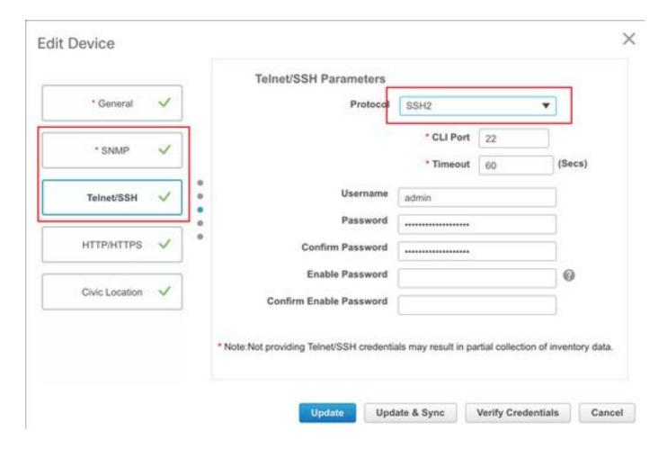
Press sync and ensure that the copy of configuration is up-todate.
