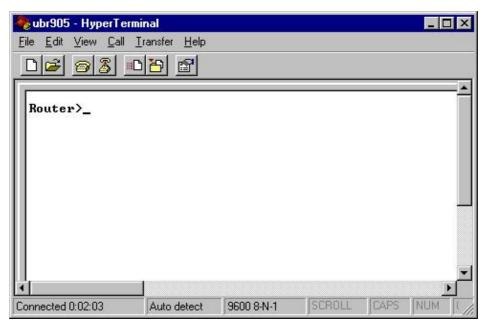
7. In order to begin configuring or performing advanced troubleshooting on the uBR900 cable modem, enter enable mode by issuing the **enable** command.
