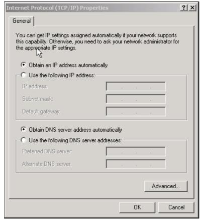
c. Ensure that the **Obtain an IP address automatically** and **Obtain DNS server address automatically** radio buttons are selected.
