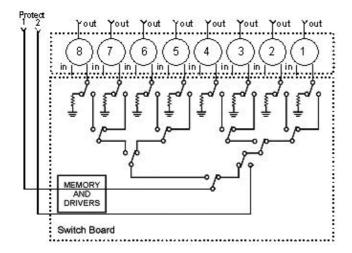
The combiner components are located in the switch chassis, but the relays are in each individual, removable module. Each relay terminates with a 75–ohm load, only in the Protect path, not the in/working path.
