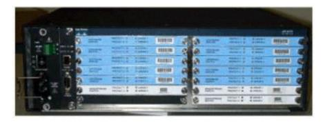
There are ten US (shown in blue) and three DS (shown in gray) modules installed in the 3x10 RF Switch. The bottom left is known as module N and is blank. The modules on the front, starting from the upper right corner, are numbers 1–13, and correlate to the ports A–M. Upstream Module 1 has all the relays for port A in slots 1 through 8 and protect 1 and 2 on the back. Module 2 is on the left and has all the relays for port H in slots 1 through 8 and protect 1 and 2.
