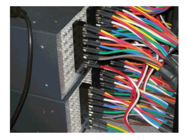
The MCX connectors can be directly attached to the switch, however, you run the risk of loose connections, emissions, and possible intermittent disconnects. Cisco developed a header to resolve these issues.
