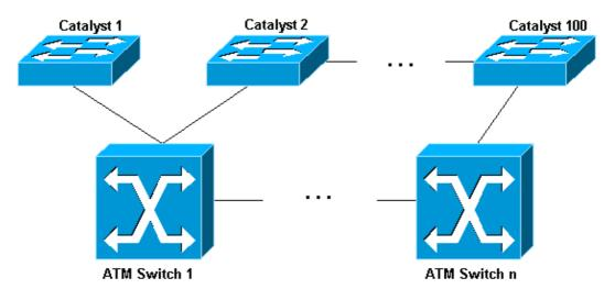
When creating the LECs on the LANE module, all LECs go up as soon as they are configured. During operation, the LES process might become overloaded, and the LANE module will run out of memory. Design 2 below solves both these problems.
